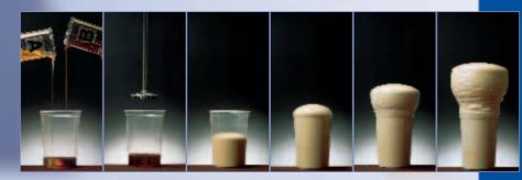
Elastopor H and Elastopir are both two or multi-component polyurethane rigid foams. When the individual components are mixed together, a reactive system is created. The foam can increase to 20 times the original volume of the two components. Aesthetic Construction Elements Shaped to Please: self-supporting sandwich elements for walls and roofs
