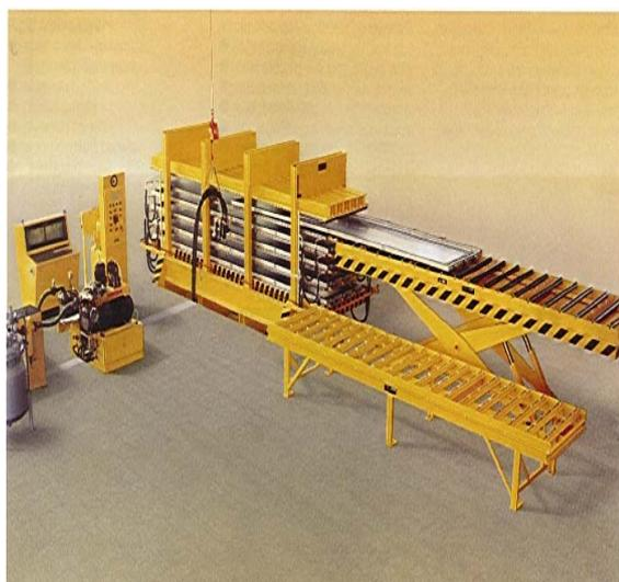
Elastopor insulation foam is produced using specially designed processing equipment capable of accurately metering the liquid components and mixing them together. The output rate of the equipment is adjustable both in terms of the rate and the ratio of the components. The weight of foam dispensed during each foam injection is controlled by a timer. Two basic types of machine are available:
