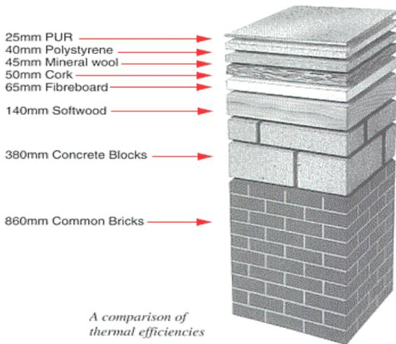
Elastopor<sup>®</sup> H - Insulation Foam is a closed cell polyurethane foam used in many applications in the field of heat and cold protection due to its excellent thermal insulation properties.
