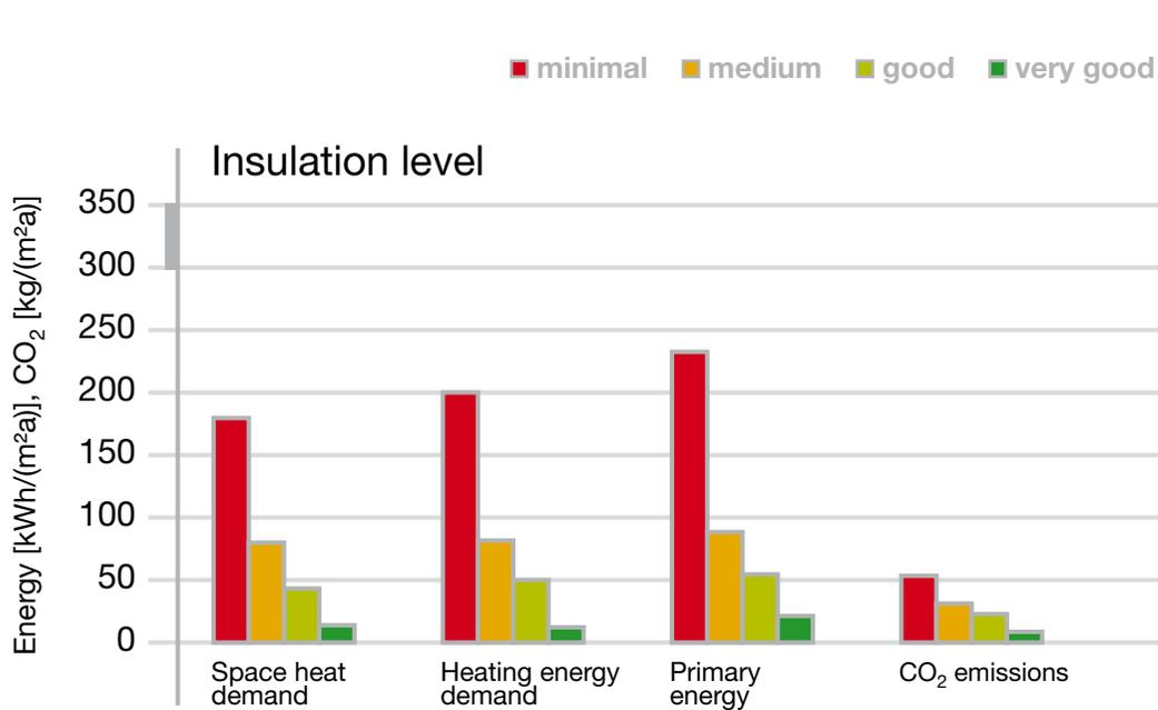
With only 15 cm roof insulation with Elastopor® H, 15 cm wall insulation made of Neopor® and 8 cm perimeter and slab floor insulation with Styrodur® C you can reduce energy consumption and CO<sub>2</sub> emissions by 75%.\*
