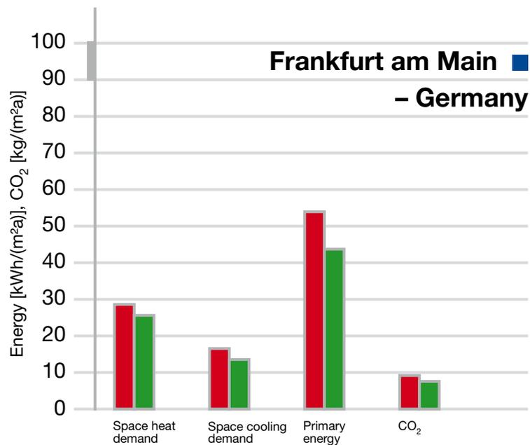
In Warsaw and Frankfurt, with SmartBoard<sup>®</sup> gypsum panels containing Micronal<sup>®</sup> PCM by Knauf, you can reduce energy consumption and CO<sub>2</sub> emissions by more than 15% and 20% respectively and significantly increase the building's comfort.
