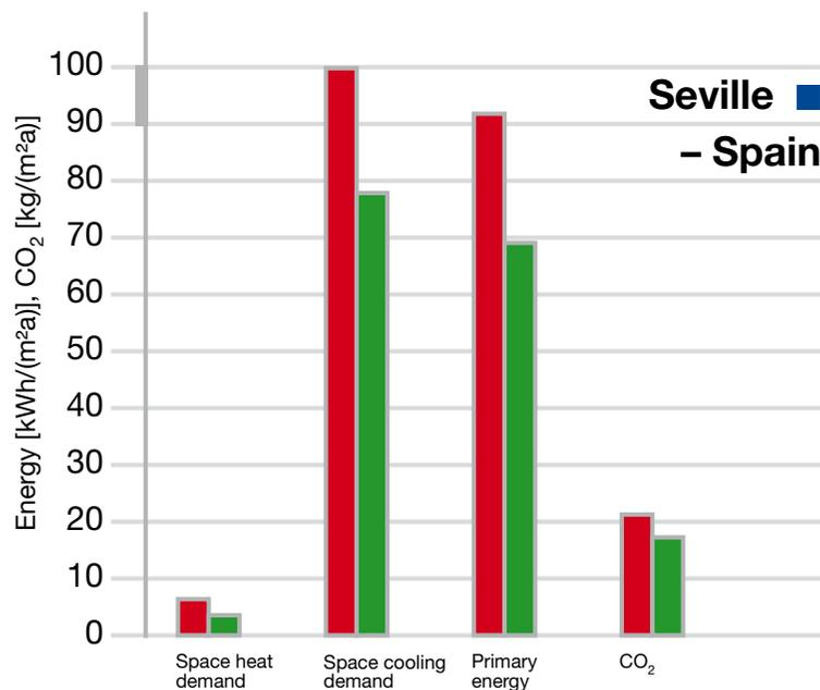
In Rome and Seville, with SmartBoard® gypsum panels containing Micronal® PCM by Knauf, you can reduce both energy consumption and CO<sub>2</sub> emissions by more than 20% and significantly increase the building's comfort, both in winter and in summer.
