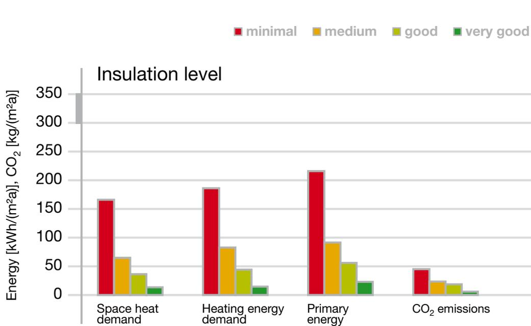
With only 15 cm roof insulation with Elastopor® H, 15 cm wall insulation made of Neopor® and 8 cm perimeter and slab floor insulation with Styrodur® C you can reduce energy consumption and CO<sub>2</sub> emissions by more than 70%.\*
