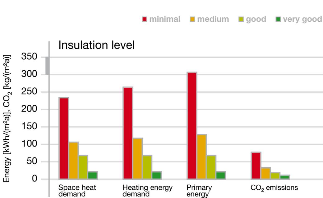
With only 15 cm roof insulation with Elastopor<sup>®</sup> H, 15 cm wall insulation made of Neopor<sup>®</sup> and 8 cm perimeter and slab floor insulation with Styrodur<sup>®</sup> C you can reduce energy consumption and CO<sub>2</sub> emissions by almost 75%.\*
