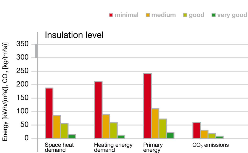
With only 15 cm roof insulation with Elastopor® H, 15 cm wall insulation made of Neopor® and 8 cm perimeter and slab floor insulation with Styrodur® C you can reduce energy consumption and CO<sub>2</sub> emissions by 70%.\*
