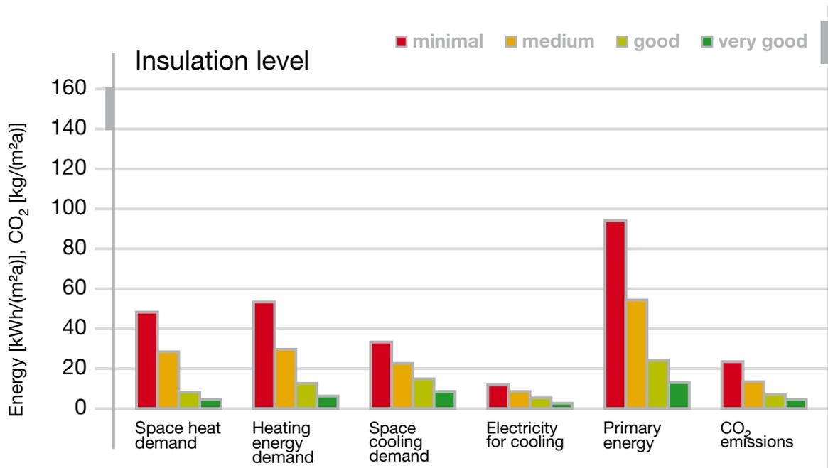
With only 8 cm roof insulation with Elastopor® H, 10 cm wall insulation made of Neopor® and 4 cm perimeter insulation with Styrodur® C you can reduce energy consumption and CO<sub>2</sub> emissions by 75%.\*
